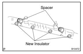
(b) Install the 2 spacers and 4 new insulators to the cylinder head.
