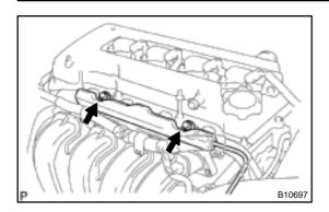
(j) Tighten the 2 bolts holding the delivery pipe to the cylinder head.
